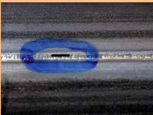
Defect in a welding seam of an aluminium tube: groove 3 x 1 x 0.3mm
